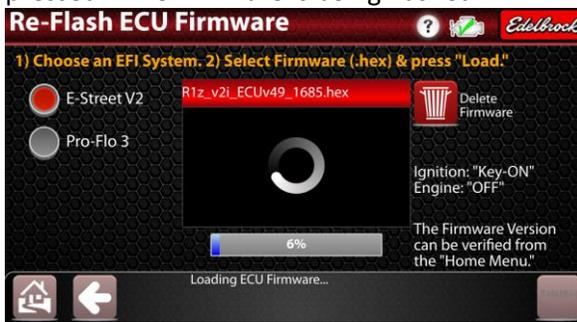
9. Once the firmware is done loading, the E-Tuner app will automatically stop the Bluetooth connection. You must now Power-Cycle the ECU for 10 seconds.
