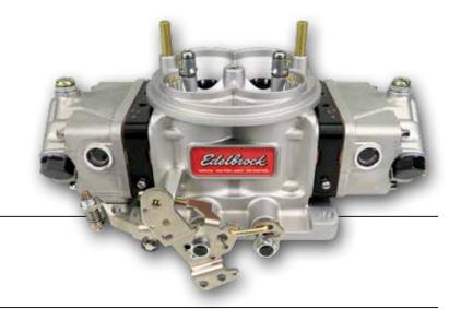
Catering to racers and street-performance enthusiasts, this new 950 CFM VRS-4150 is calibrated for E85 ethanol-fueled vehicles. Custom four-circuit billet metering blocks and extra-large fuel jets, specifically designed for E85, flow 30% more fuel than a conventional 950 VRS while maintaining all the convenient features not usually found in a racing carburetor.
